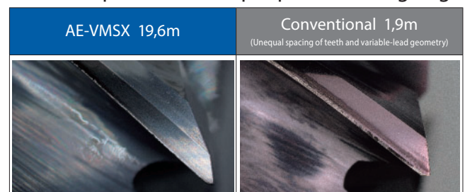
Wear comparison of the peripheral cutting edge
